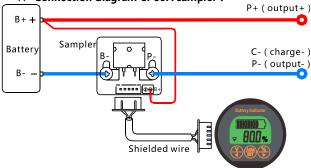
★ Connection diagram of 100A/350A sampler :
